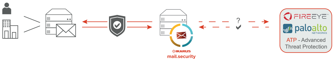
Fig. 1 - IKARUS mail.security scans all incoming and outgoing emails before they reach your network. The sandboxes by FireEye and PaloAlto can optionally be switched on.
